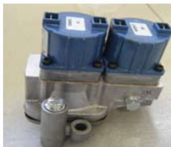
CONTROL VALVE AT2E-1806-2 - NG (5"WC) AT2E-1806-3 - P (10"WC)
