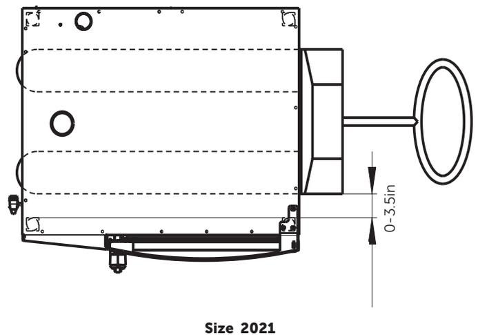
FIGURE: 9 Handling by a fork-lift stacker
