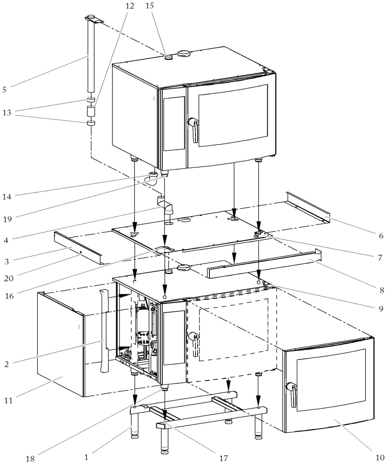
FIGURE: 28 Two comboven arrangement.
