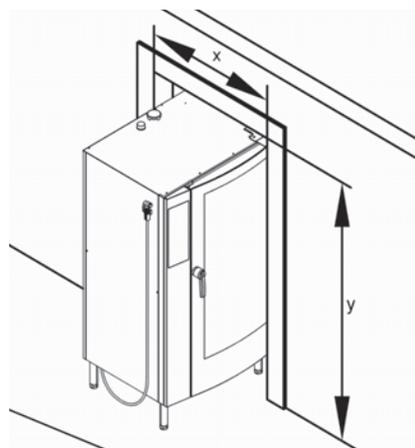
FIGURE: 7: Check required dimensions of door.
