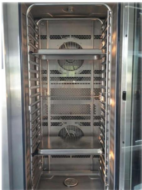
FIGURE: 27 Ovens with one fan, only need one pan. In the case of units with 2 fans, two hotel pans must be inserted, to properly calibrate unit
